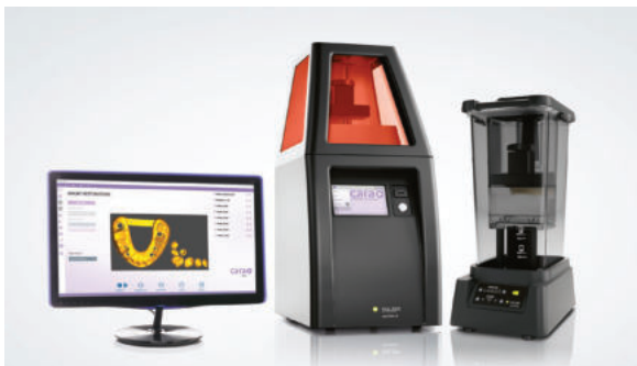
Figure 15: With the help of 3D-print technology, the design data was used to print the prosthesis structure in the cara Print 4.0 unit out of a tooth-coloured acrylic.
