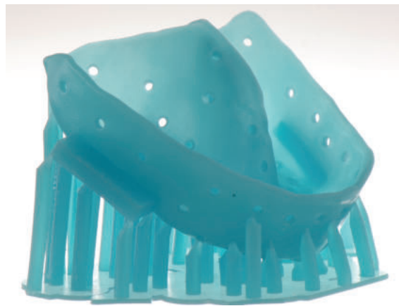
Figure 7: The individual impression tray for an open impression was optimized with open source-software using the digitized surgical template and printed in the 3D printer.
